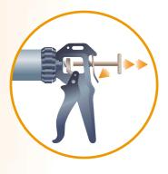
A Press lever clasp release and pull pressure piston out to maximum position.
